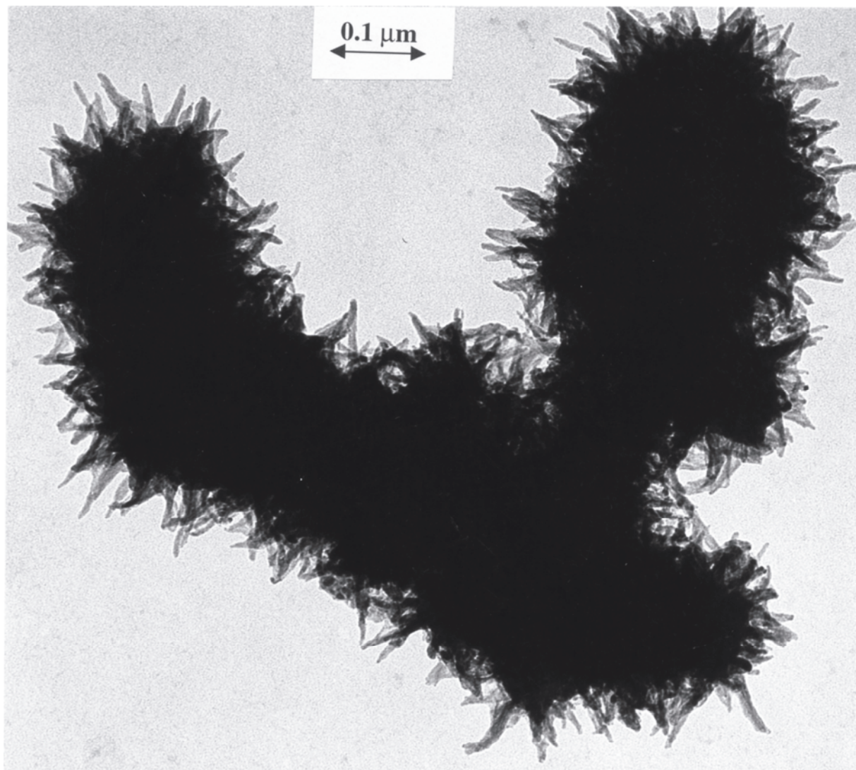
Figure 7. Transmission electron microscopy (TEM) photomicrograph of synthetic schwertmannite.
